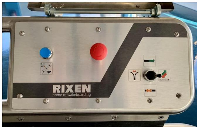
By activating the ready-loading function, the ball rope in the magazine is pushed forward from the pre-loading position. The line is loaded ready and the next carrier takes the tow-rope with it.
